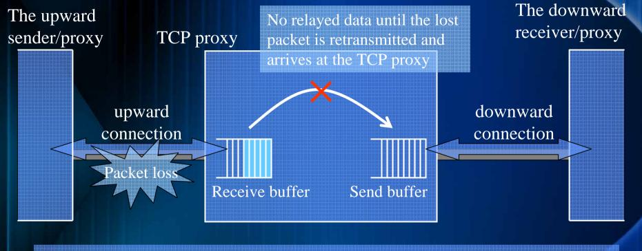
The send buffer of downward connection becomes empty and downward connection cannot send packets to the downward receiver/proxy.
