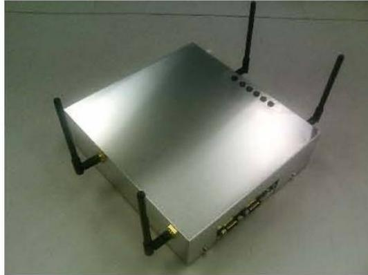
Figure 24: The ad-hoc wireless relay node (Hitachi Information & Communication Engineering).
