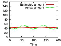
(c) Traffic between nodes 2 and 14 (case of using Eq.(3.26) with  $\Phi{=}0.01)$
