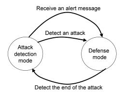
Figure 2.26: State transition diagram between attack detection mode and defense mode
