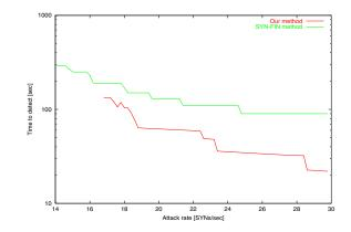
Figure 2.12: Time to detect attacks with our method and with SYN-FIN method
