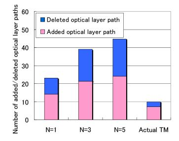
Figure 3.7: Number of added/deleted optical layer paths of additional equation method
