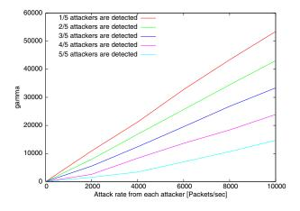
Figure 2.21: Relationship between attack rate and  $\gamma$  to identify attachk sources
