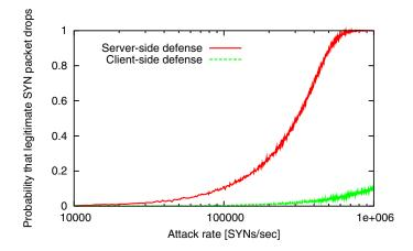
Figure 2.35: Probability of dropping legitimate SYN packets vs. attack rate
