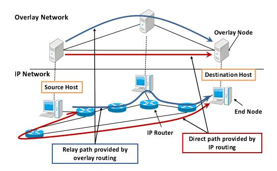
Figure 1: Overlay routing
