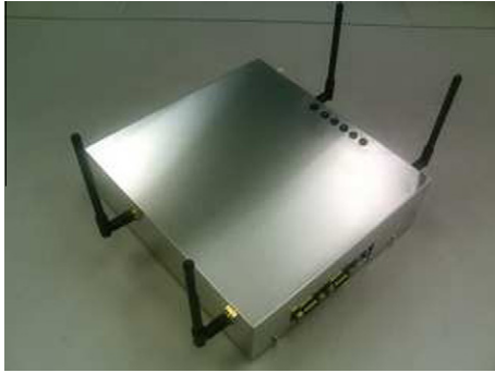
Fig. 12. The ad-hoc wireless relay node.
