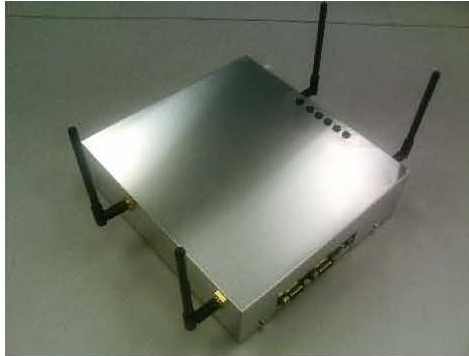
Figure 2.12: Ad-hoc wireless relay node
