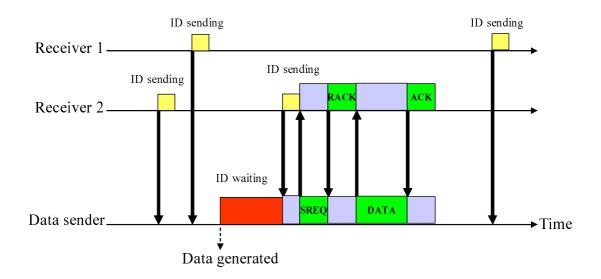
Figure 2: Data transmission process in the IRDT protocol
