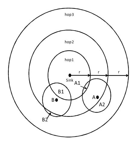
Figure 1: Forward and backward node numbers deviation problem due to topology. For node "A", forward node area is "A1", backward node area is "A2". For node "B", forward node area is "B1", backward node area is "B2".
