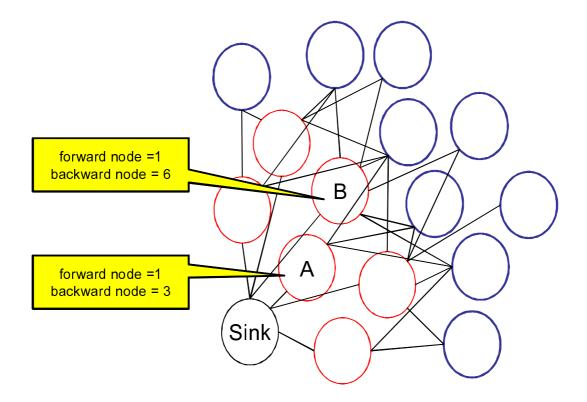
Figure 6: Packet relaying load difference at nodes. Red nodes are in hop 1, Blue nodes are in hop 2.
