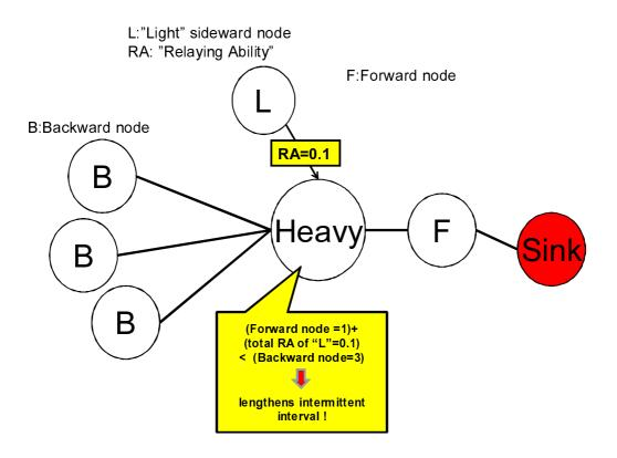
Figure 10: "Heavy" node lengthens the intermittent interval
