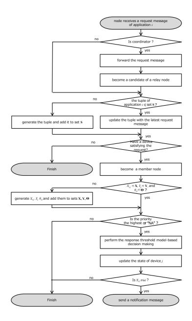
Figure 7: Behavior of a node on receiving a request message
