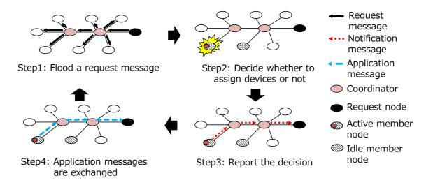
Figure 6: Overview of device assignment
