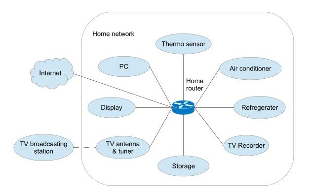
Figure 5: Overview of home device control system
