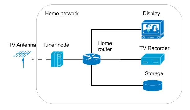
Figure 6: Network overview of TV's peripheral equipment using CCN
