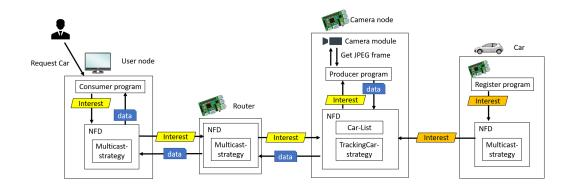
Figure 4: Component diagram of tracking system
