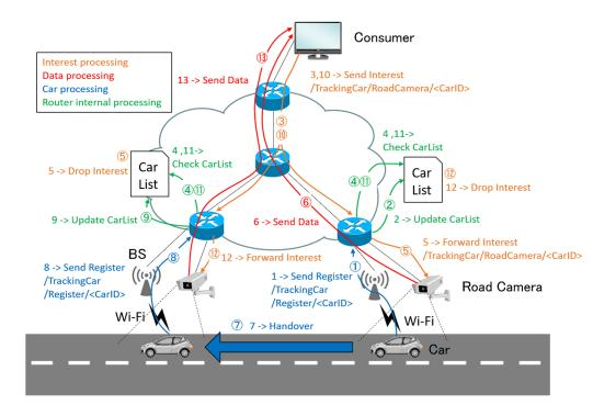
Figure 3: Communication procedure of Tracking System for moving objects
