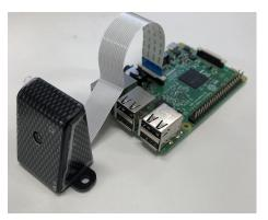
Figure 10: Raspberry Pi 3 Model B
