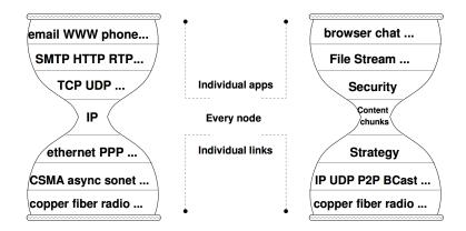
Figure 1: Protocol stacks of IP networking and NDN (cited from [1])
