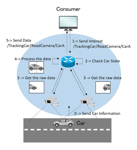
Figure 8: Overview of system utilizing in-network processing
