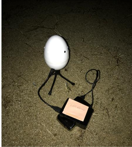
Figure 4: Raspberry Pi 3 Model B with an 8-channel microphone array (TAMAGO-03)
