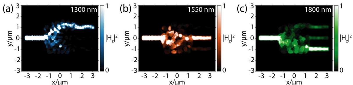
**Fig. 2.** Calculated magnetic field intensity distributions at the wavelengths of (a) 1300 nm, (b) 1550 nm and (c) 1800 nm for the firstly designed wavelengths demultiplexer device.
