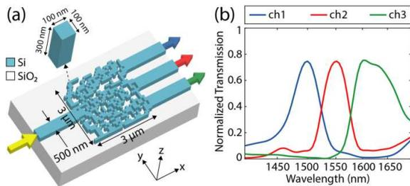
**Fig. 3.** (a) Perspective view of designed device for demultiplexing the wavelengths of 1500 nm, 1550 nm, 1600 nm) with its structural parameters and (b) plots of normalized transmission efficiencies at the output waveguides. Same colors are used for arrays at output waveguides and corresponding calculated transmission efficiencies.
