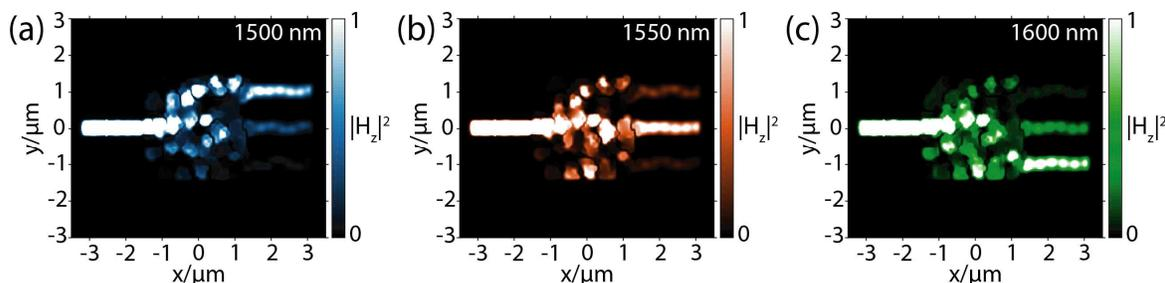
**Fig. 4.** Calculated magnetic field intensity distributions at the wavelengths of (a) 1500 nm, (b) 1550 nm and (c) 1600 nm for the secondly designed wavelengths demultiplexer device.
