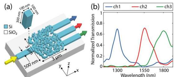
**Fig. 1.** (a) Perspective view of designed device for demultiplexing the wavelengths of 1300 nm, 1550 nm, 1800 nm) with its structural parameters and (b) plots of normalized transmission efficiencies at the output waveguides. Same colors are used for arrays at output waveguides and corresponding calculated transmission efficiencies.
