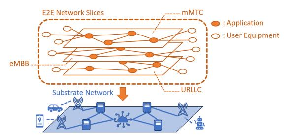
Figure 1: Diagram of E2E network slicing in 5G network
