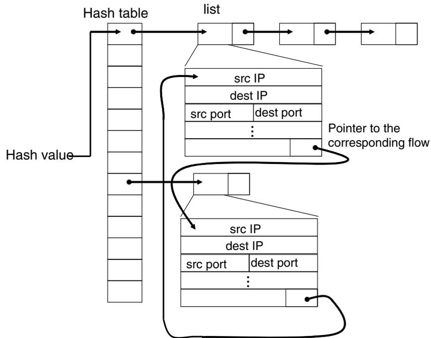
Figure 2.30: Data structure to hold normal flows
